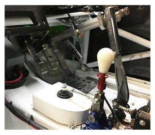
Firstly fully remove your cars original mechanical handbrake system if fitted (Unless The Car Requires an MOT). – The hydraulic handbrake is not for permanent parking use.
