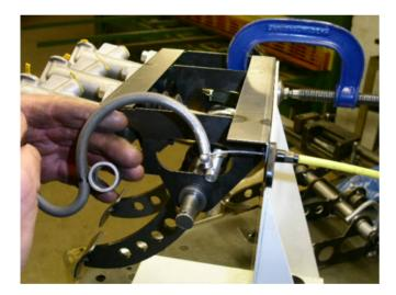
Slot the ball of the cable into the drilled hole in the pedal.
